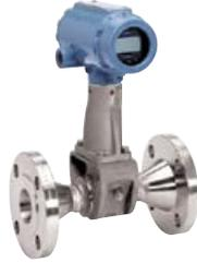
The Rosemount 8800 Reducer Vortex flow meter handles lower flows better than any other Vortex meter. The common face-to-face dimension allows you to change the meter without impacting the piping layout.
